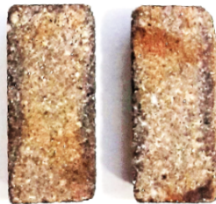
Figure 8: Along the axis cut of the core Bent2 after treatment following the static aging protocol. The darkened areas at the outer part of the core are asphaltene and resin deposits.
