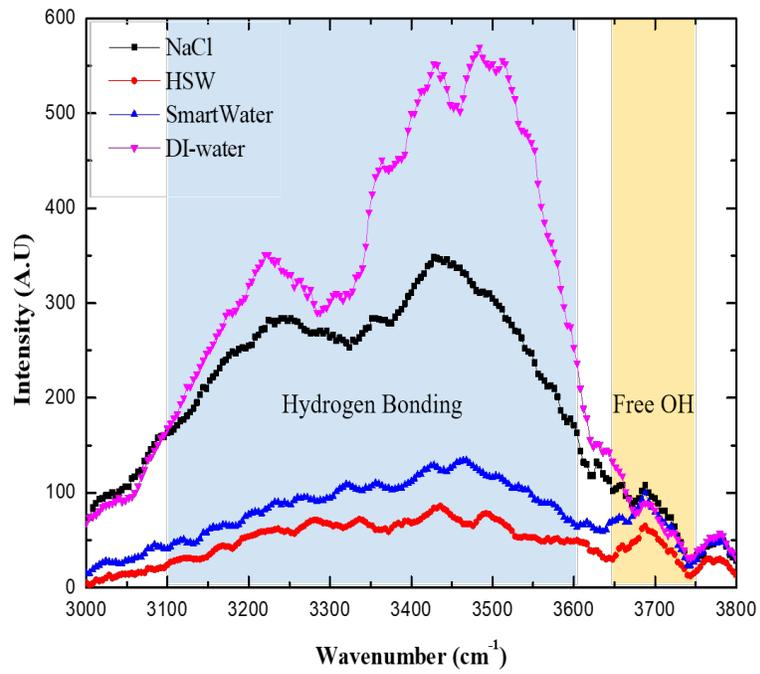
**Figure 6.** Hydrogen bonding and free OH behaviors at n-dodecane/SA/brine interfaces
