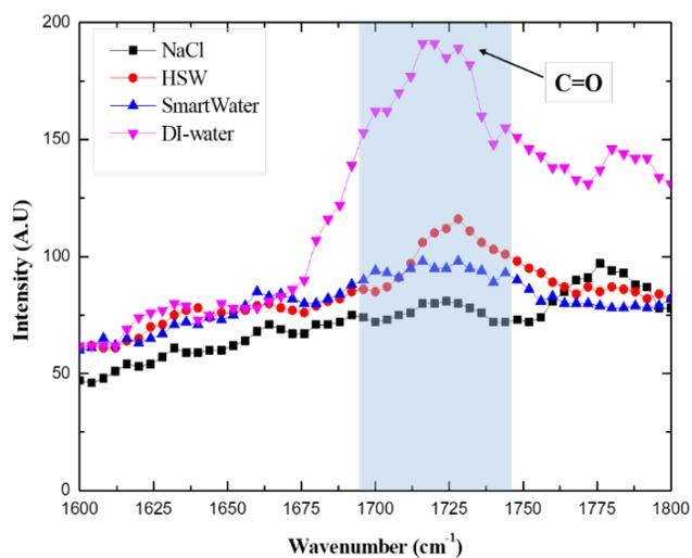
**Figure 4.** The C=O intensities of different brines at oil/water interfaces
