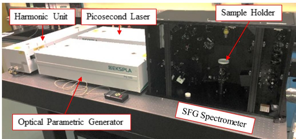
**Figure 1.** Sum Frequency Generation Spectrometer Setup
