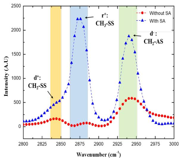
**Figure 3.** The carboxylic acid effects on the SFG intensities of n-dodecane/DI-water
