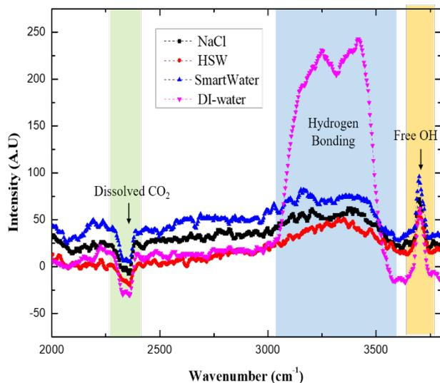
**Figure 2.** SFG results of different brines at air/water interfaces.
