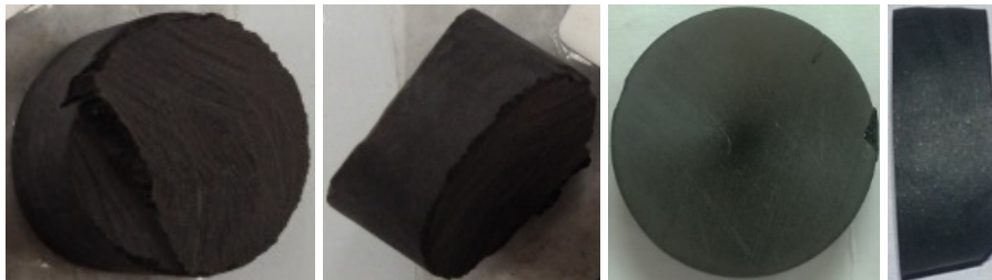
Figure 1. Photos of the SL5 sample, cylinder diameter 2.5 cm. Left to right: top view before pre-processing, side view before pre-processing, top view after pre-processing, side view after pre-processing.
