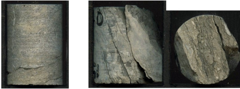
Figure 3: Oilfield S. Damaged Dean Stark plug (left) and damaged Hot Shot Plug (right). after cleaning and drying. Sample diameter is 1.5" inch.
