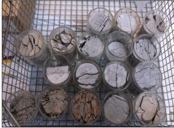
Figure 2: Damaged RCA plugs from oilfield S after cleaning and drying. Sample diameter is 1.5” inch.
