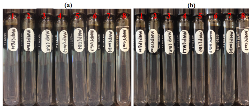
Figure 12 FNP-MD suspensions stability screening with different type of oils: (a), Day 1; (b), Day 30; (1: PEN; 2: TMB; 3: BR; 4: ML; 5: TB; 6: VG; 7: WD; 8: Decane).
