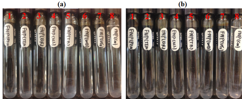
Figure 11 FNP suspensions stability screening with different type of oils: (a), Day 1; (b), Day 2; (1: PEN; 2: TMB; 3: BR; 4: ML; 5: TB; 6: WD; 7: VG; 8: Decane).
