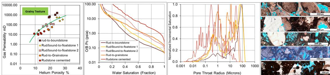
Figure 8 Rudstone 5 RRT's: representative MICP curves and thin-section photomicrograph are given for each RRT
