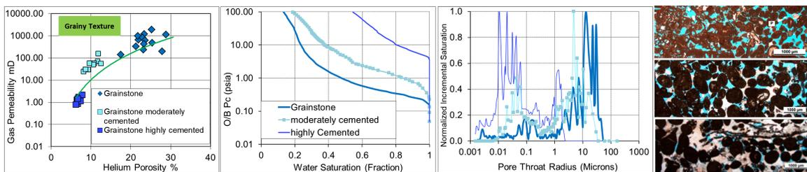
Figure 7 Grainstone 3 RRT's: representative MICP curves and thin-section photomicrograph are given for each RRT
