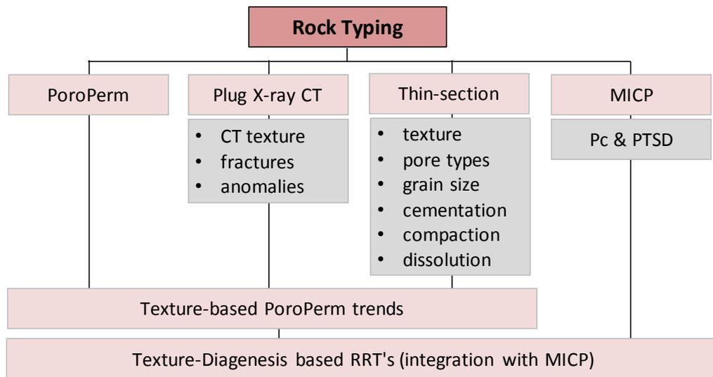
Figure 1 Workflow of the Rock Typing approach followed in this study
