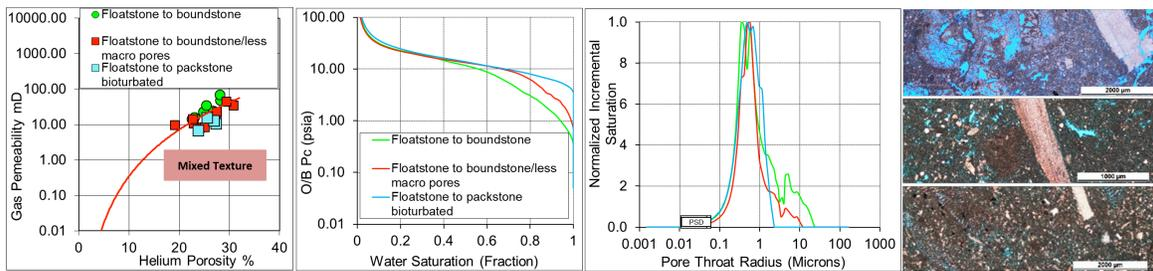
Figure 11 Floatstone 3 RRT's: representative MICP curves and thin-section photomicrograph are given for each RRT
