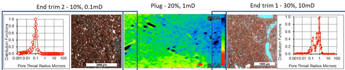
Figure 2 In the middle is shown a color-scale plug CT image with 20% porosity and 1mD. End trim 1 was cut from the right end of the plug and gave very different geological and petrophysical data from the end trim 2, which was cut from the left side. This shows the importance of the plug CT image.
