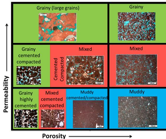
Figure 4 Texture-Diagenesis PoroPerm Diagram
