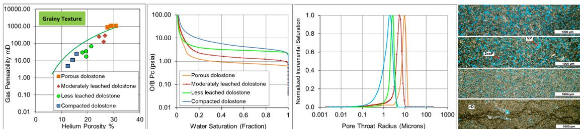
Figure 9 Dolomitic 4 RRT's: representative MICP curves and thin-section photomicrograph are given for each RRT
