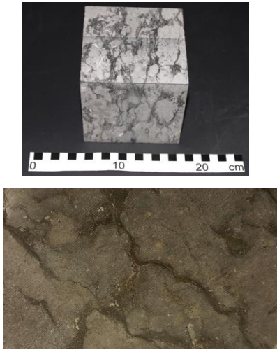
Figure 1. The visual heterogeneity of the Cobourg limestone (top) cuboid measuring 300 mm (bottom) modular regions in a zone measuring 100 mm x 130 mm
