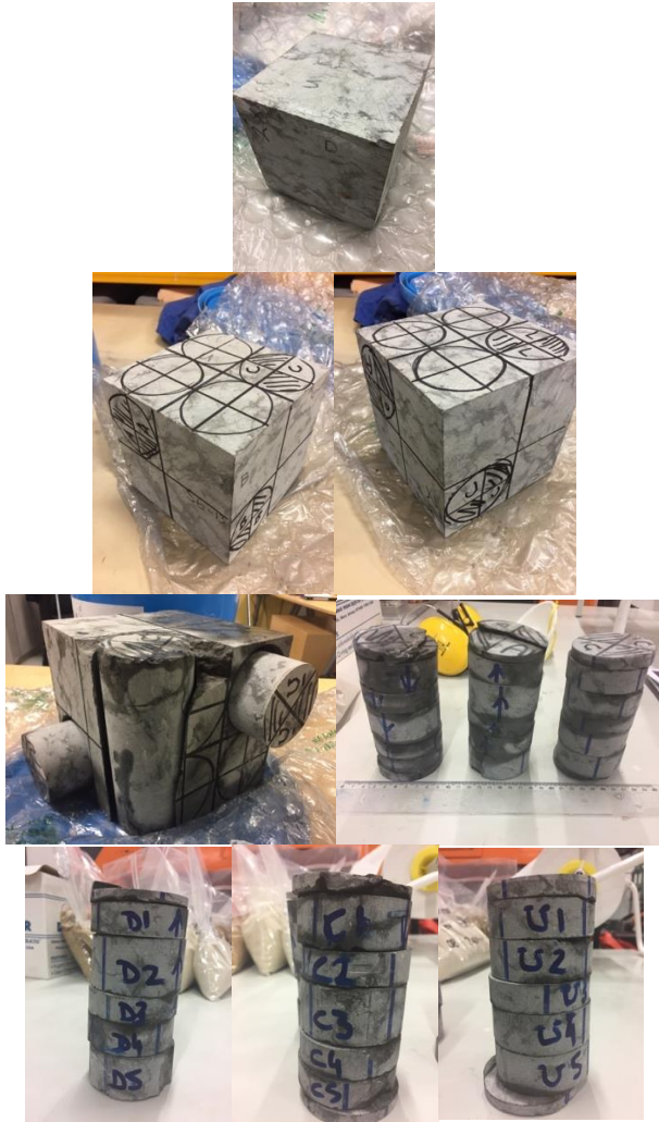
Figure 4. Sample preparation from a cube provided by Mc Gill University to cylinders of 65 mm diameter and varying height
