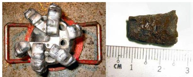
**Fig. 4.** MCB and one of the micro-cores collected while drilling an interbedded shale and sandstone formation [18]
