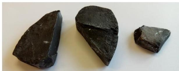
**Fig. 5.** Pieces from a broken shale core having irregular forms and too small sizes to be plugged
