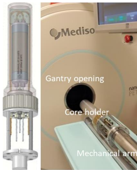
Fig. 5. A custom-made core holder by RS systems © (Trondheim, Norway) is installed on a mechanical arm for imaging with high-resolution PET.
