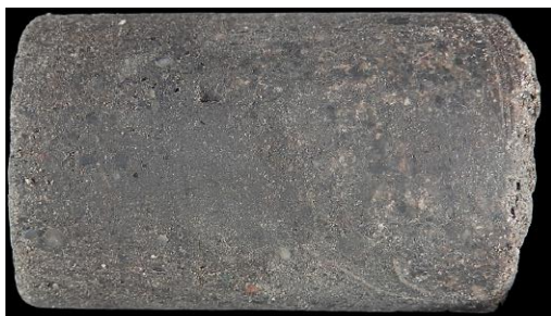
Fig. 15. Side view in white light photo of siliciclastic RSWC (wellbore end on the left side).
