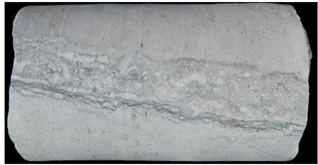
Fig. 12. Side view in white light photo of carbonate RSWC (wellbore end on the right side).
