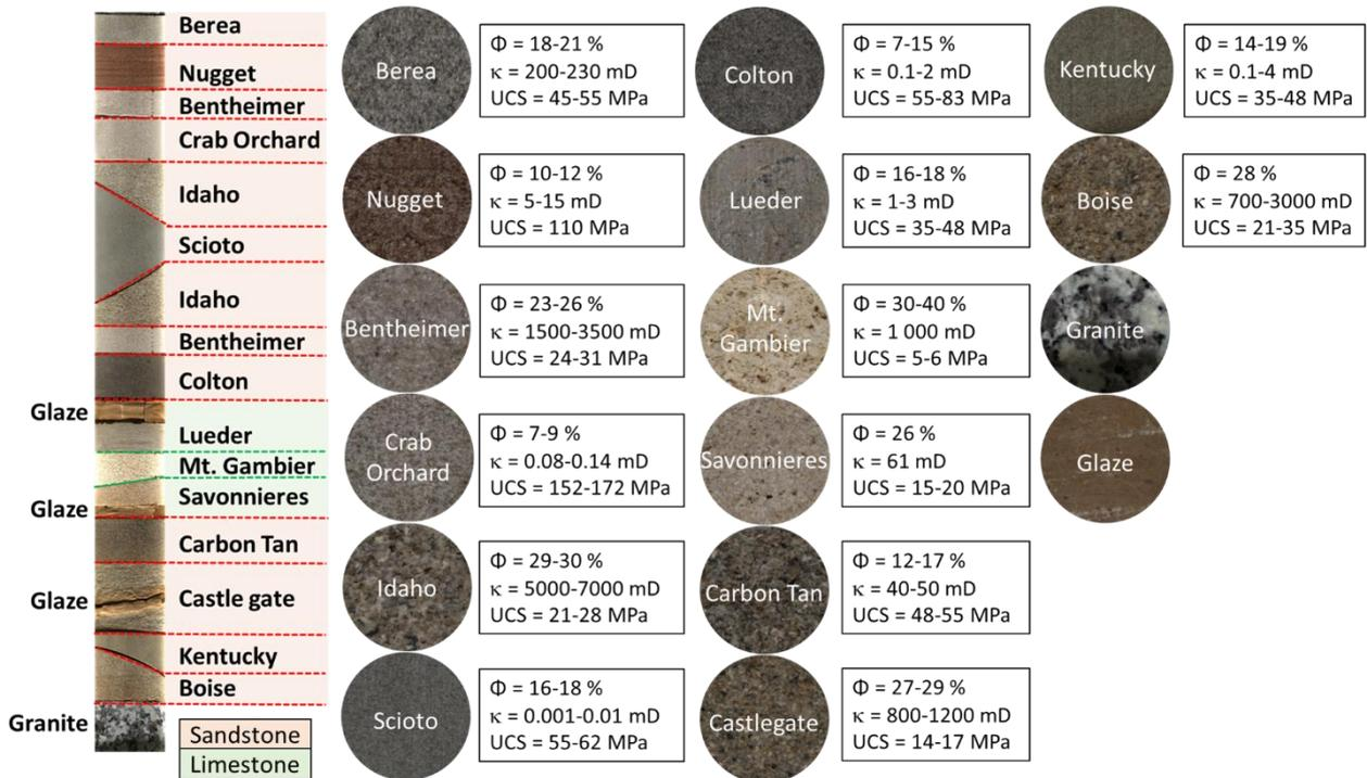
**Fig. A1.** Composite core and description of the analogue sandstones and limestones used to create the core. The porosity, permeability and uniaxial compressive strength (UCS) reported here are the ones provided by the rock suppliers or extracted from the literature [10, 11,12]
