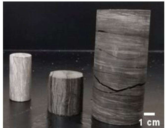
Fig. 1. Mancos Shale samples. Different colors refer to compliant (dark) and stiff (light) layers.
