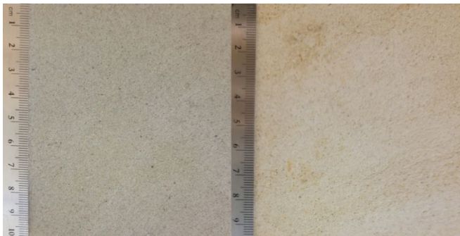
Fig. 4. Homogeneous rock samples. Berea Sandstone (left) and Texas Cream Limestone (right).
