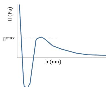
Fig. 5 Schematic of a disjoining pressure isotherm
