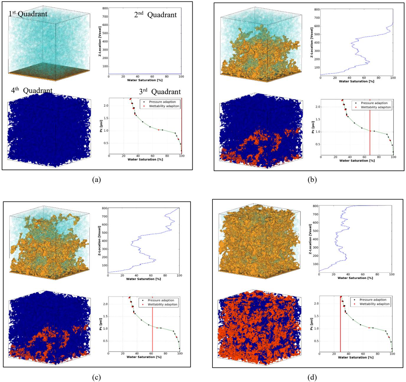
**Fig. 7.** Various stages of wettability alteration simulation. The 1<sup>st</sup> quadrant in each figure shows an iso surfaces of oil (beige) and a volume rendering of water (blue), 2<sup>nd</sup> quadrant shows the water saturation profile along the flow direction, 3<sup>rd</sup> quadrant shows capillary pressure versus water saturation chart and 4<sup>th</sup> quadrant shows oil wet (red) and water wet (blue) surface within the pore space in 3D.
