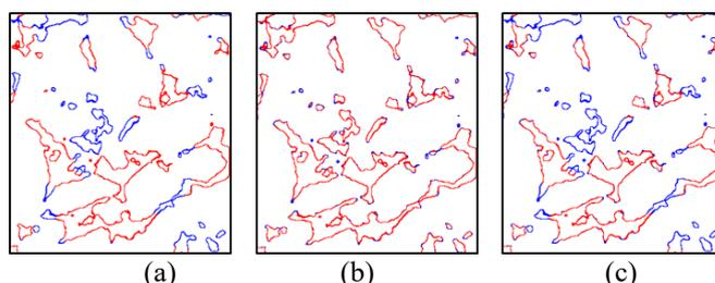
Fig. 6. Surface selection (red) for wettability alteration: (a) selection is adjacent to a non-wetting phase, (b) selection satisfies  $P_c > P_v + \Pi^{max}$  condition and (c) selection is subset of (a) and (b).
