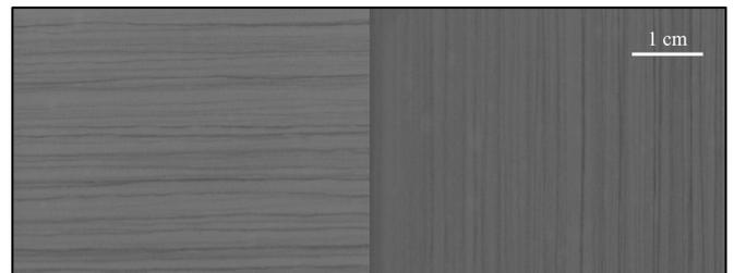
**Fig. 3.** X-ray radiographs of a laminated rock sample cut with bedding planes parallel (left panel) and perpendicular (right panel) to flow, respectively.
