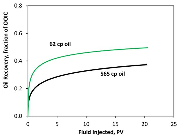
Fig. 5. Calculated (Buckley-Leverett Equation) oil recovery curves for 565 cp and 62 cp oils.
