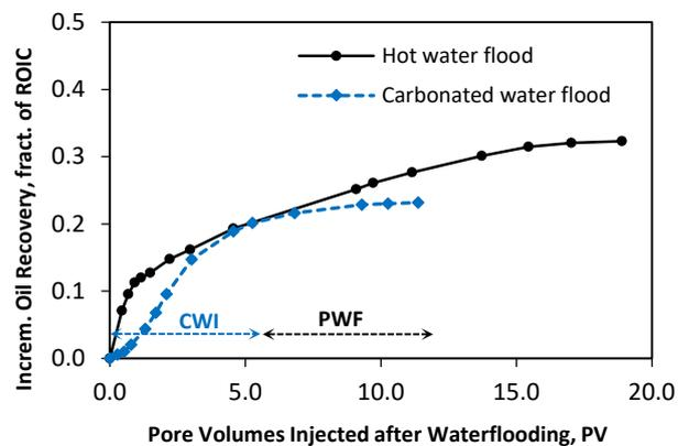
Fig. 6. Incremental oil recovery as functions of pore volumes injected after waterflooding. ROIC—remaining oil in core after waterflooding; CWI—carbonated water injection; PWF—post water flush.
