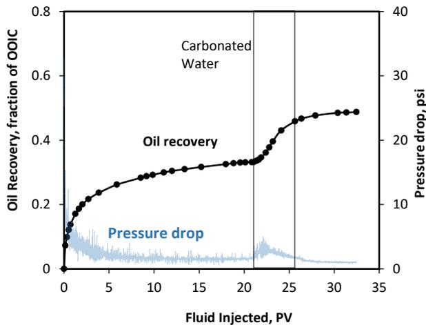
**Fig. 1.** Oil recovery and pressure drop as functions of injected pore volumes. Carbonated water flooding.
