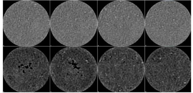
**Fig. 2.** Comparison of CT images before and after carbonated water flooding. The first row were four consecutive CT images scanned on the core plug before coreflooding, and the second row showed the corresponding images obtained after the coreflooding test. The left side image was the inlet face CT slice.
