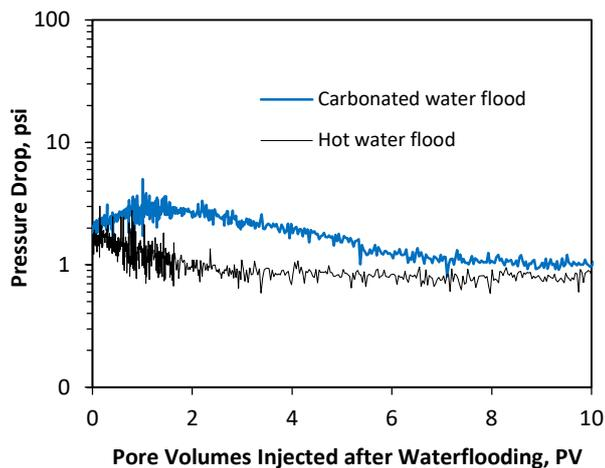
Fig. 7. Pressure drop as functions of pore volumes injected after waterflooding.
