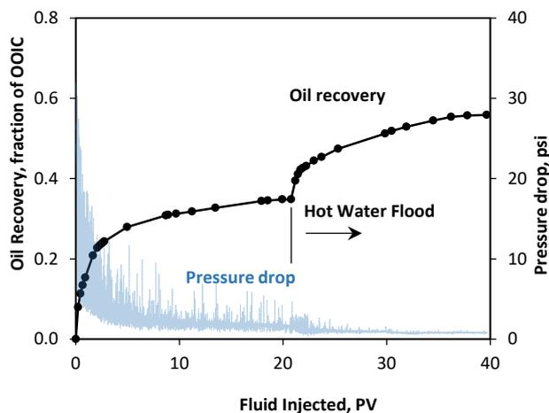
Fig. 4. Oil recovery and pressure drop as functions of injected pore volumes. Hot water flooding.
