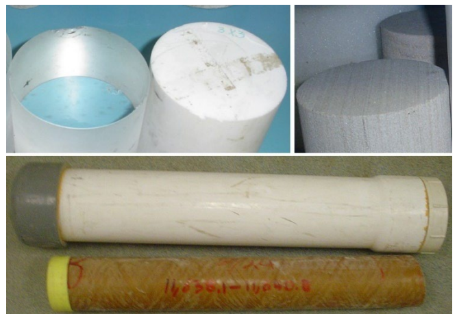
Fig. 4. Calibration ‘standards’ - quartz, Macor, Berea and a representative cleaned sandstone (top). Blank PVC core box and fiberglass core sleeve (bottom).
