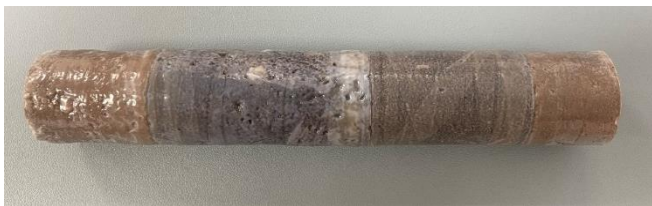
Fig 6: Core plugs were put together to make the composite core for the experiments
