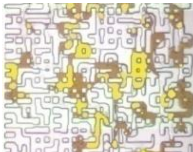
Fig. 5. CO 2 dissolves in the oil phase, a new gas phase is formed spontaneously within the oil phase during CWI.
