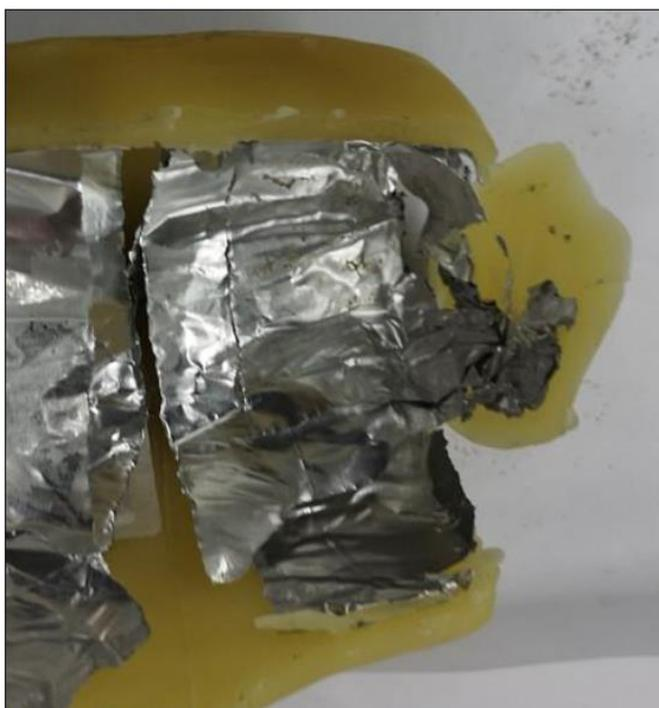
**Figure 5.** Degraded aluminum wrap from a UAE wax preserved core plug sample.
