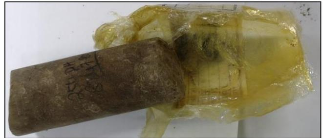
Figure 2. Crude oil penetrated the LDPE cling film of this RP40<sup>[15]</sup> wrap/wax preserved sample after several years storage. The rock sample was dry to the touch.
