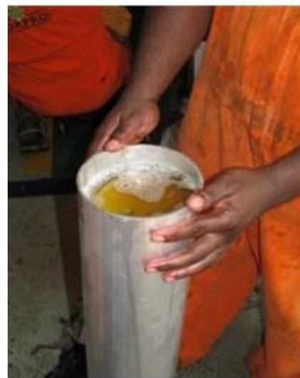
**Figure 9.** Shale whole core immersed in mineral oil. This is a very effective preservation technique for preventing water loss.
