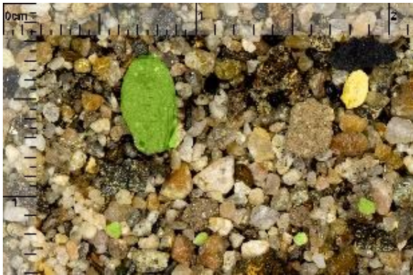
Figure 9 : grain segmentation with Mask R-CNN on a downscaled photograph of cuttings, courtesy of Stratum Reservoir.
