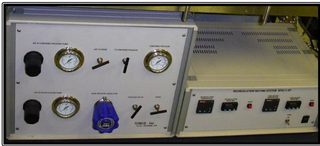
Fig. 2. Photograph of a recirculating heating system (right) with backpressure regulator and confining pressure regulator (left).
