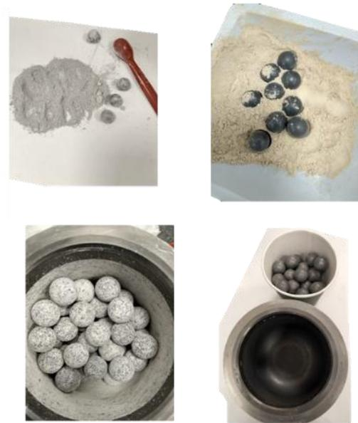
Fig. 5 Sample grinding with a mill machine; (Top, Bottom Left) ILST and (Top, Bottom Right) FBST.
