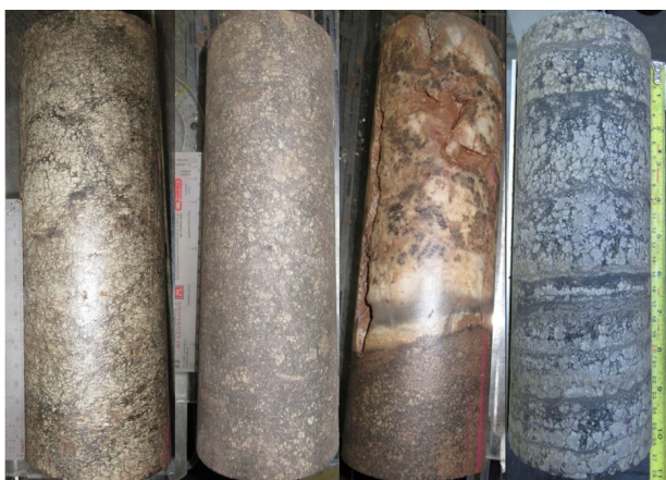
Fig. 2. Pre-salt carbonate (dolomitic-Limestone on the left, and silicified carbonate and argillaceous carbonate on the right).
