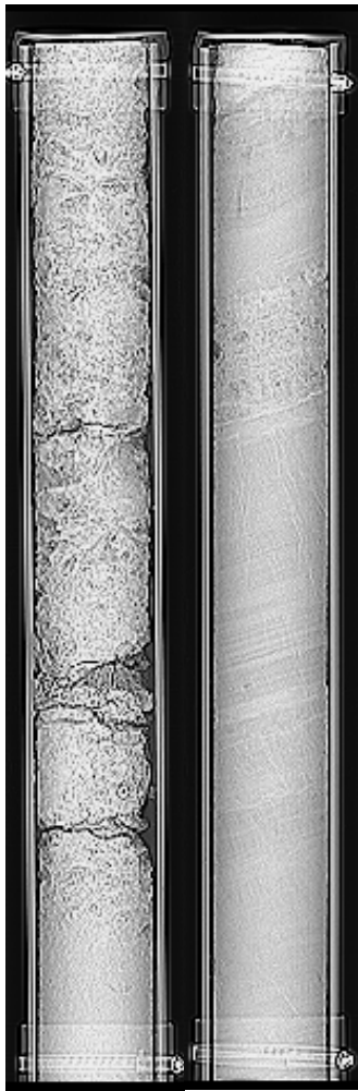
Fig. 4. Two pilot scans of whole core samples placed in 3-foot aluminium barrels. The left sample is an example of a poorly recovered sample or damaged sample. In contrast, the one on the right shows good recovery with an indication of inclined formation bedding and lamination.
