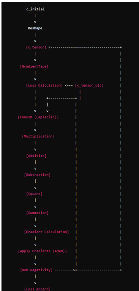
Fig. A1. Computational graph for the neural network used in place of finite difference scheme.
