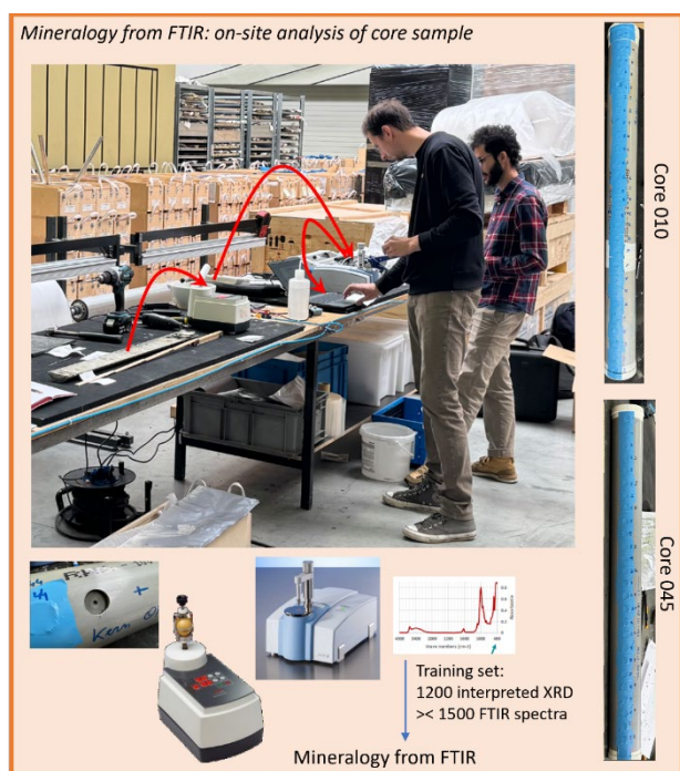
Fig.2 On-site FTIR characterization of core material of the Essen-1 and ON-Mol-2D borehole in the core repository of ESV Euridice in Mol, Belgium. Samples are either drilled using a Forstner drill of 2cm diameter from open, slabbed core (large left picture) or from closed core through the pvc tubing (lower left image). Samples are subsequently milled using a small milling device (lowermost image), measured with a Bruker Alpha-II FTIR-ATR (lower central image) and subsequently interpreted by the automated HSMQ software.
