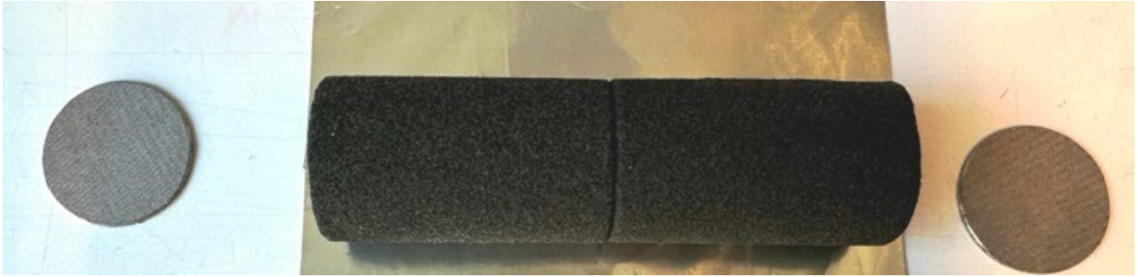
Fig. 2 Core assembly for sample CF1 to the left (inlet), and sample CF2 to the right (outlet). Adjacent to the core samples are the two filters with a 40 μm mesh size.
