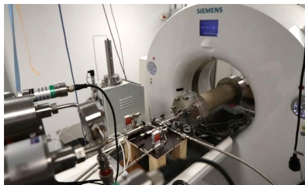
Fig. 2. Image of the core flooding setup placed on the CT scanner table.
