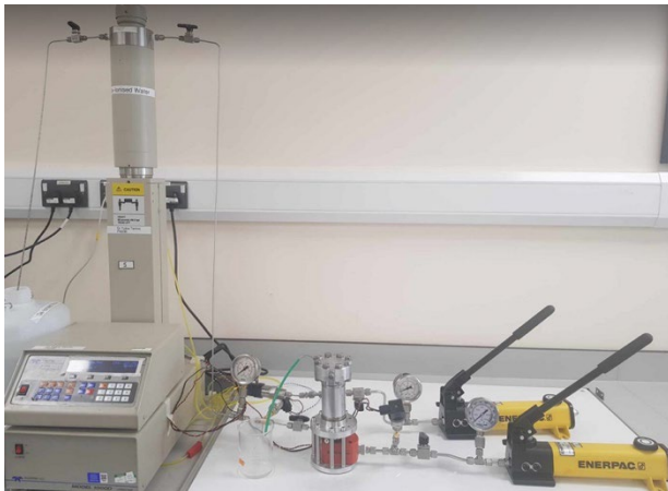
Fig. 3. Image of the fracturing and flow measurement experimental apparatus.
