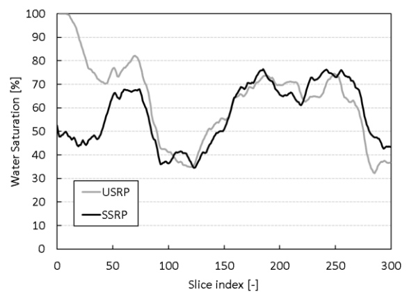
Fig. 8. Water saturation profile of 300 3 voxels subset of Berea sandstone at residual saturation of steady state relative permeability (SSRP) and unsteady state relative permeability (USRP).
