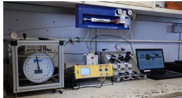
Fig. 5. De-pressuring and evolved gas monitoring system.
