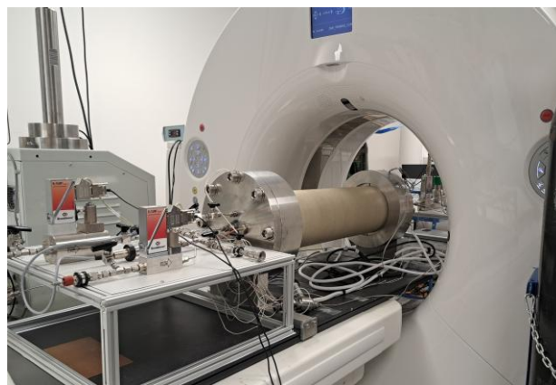
Fig. 2: Image of the core flooding setup placed on the CT scanner table
