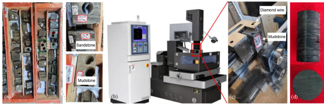
Fig. 1. Sample preparation: (a) Samples selection with different depths and lithologies; (b) Diamond wire cutting machine; (c) Rock cores processing; (d) Samples after processing.
