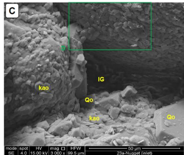
Figure 122: SEM (Scanning Electron Microscopy) Image of Nugget Sandstone Inlet Face Trim, Post Relative Permeability Testing Showing Unnaturally Oriented Platelets. Kao (Kaolinite), IG (Intergranular), Qo (Quartz overgrowth)
